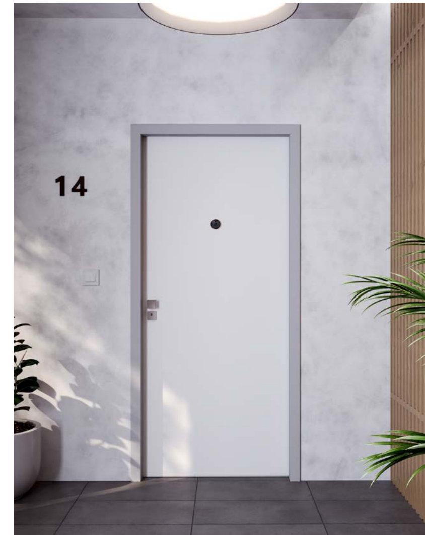
exterior view: ELEGANT 10 - HPL Antifinger premium white W1000 / SAP 865 metal doorframe in RAL 7035, fire resistance 45 min., security class RC3, acoustic rating 37 dB, climate III, M9 security hardware, Eques VEIU Pro digital door viewer
