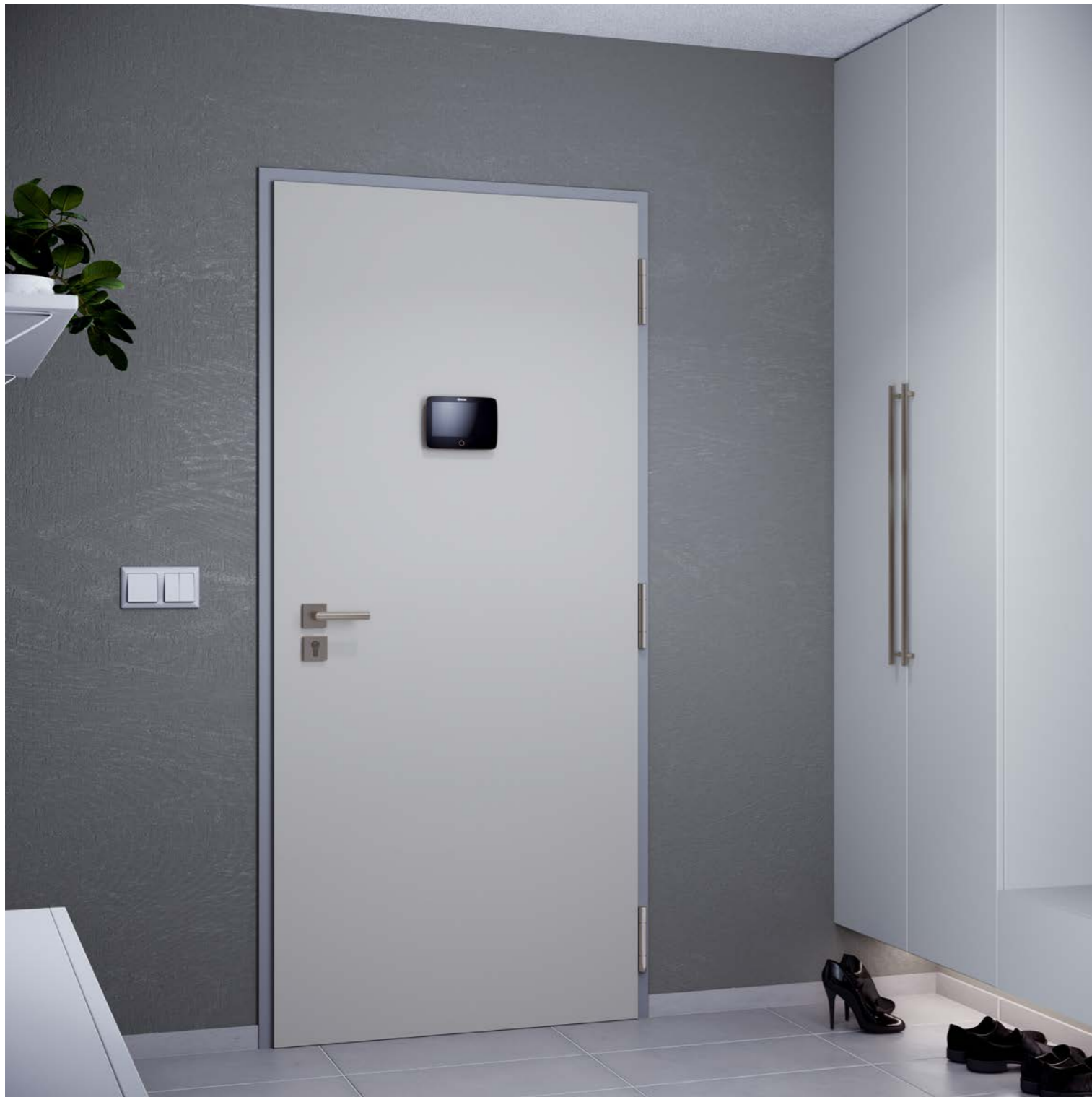
interior view: ELEGANT 10 - HPL Antifinger light grey U708 / SAP 865 metal doorframe in RAL 7035, fire resistance 45 min., security class RC3, acoustic rating 37 dB, climate III, M9 security hardware, Eques VEIU Pro digital door viewer
